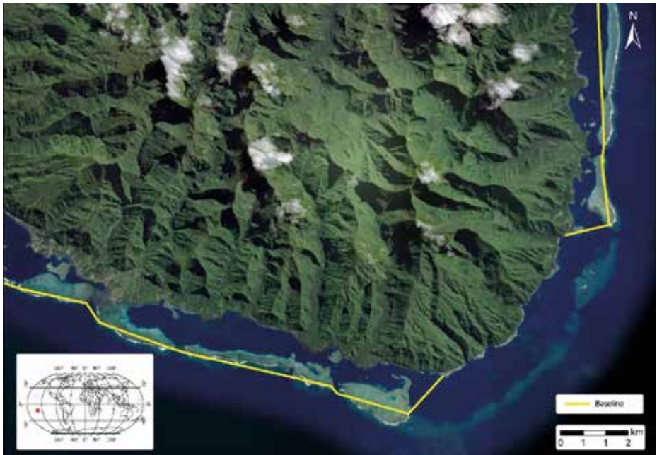
Figure 5: Detail of baseline around fringing reefs and connecting to the shoreline of the island of Tahiti, French Polynesia 67
